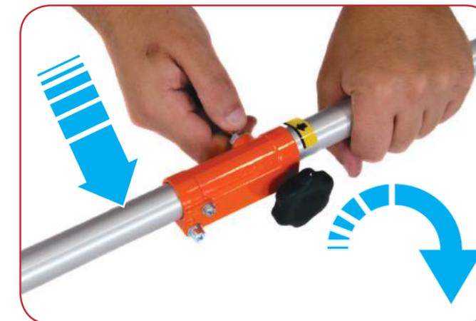
Release the pin and rotate the lower shaft until the joint is locked into position.
