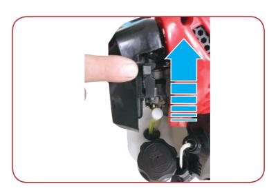
For cold engine starts close the choke by sliding the lever upwards.
