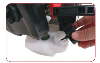
Remove the fuel cap and fill the tank to no more than 80% capacity.
