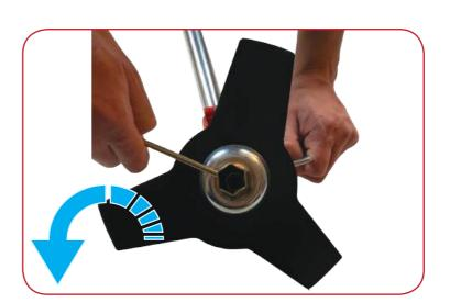
Lock the axle by placing the allen key inside the locating hole of the collar and tighten the locking nut using the wrench provided, turning anti-clockwise until secured tightly.
