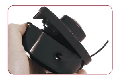
Repeat steps 2 & 3 for the second winding and thread back through the eyelets. Securing the cover by repeating 'Step 1' in reverse.
