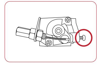
When the engine tends to stop frequently at idling mode, turn the idle speed adjuster clockwise.
