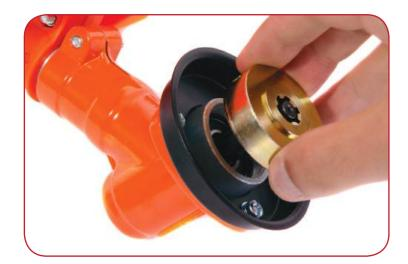
Install washer "A" as illustrated above. Align the hole in the washer with the hole in the spool collar.
