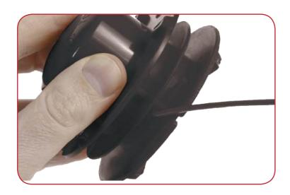
The cartridge consists of two windings which need to be wound in the direction shown on the body. Secure the replacement wire to the cartridge as shown.
