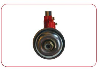
The locking washers may come pre-installed on the hub of the machine.
