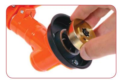
Install washer "A" as illustrated above. Align the washer with the hole on the spool collar.
