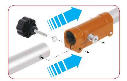
Insert the locking knob into the shaft connector.
