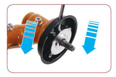
Lock the axle by placing the allen key inside the locating hole of the collar, through washer "A" and into the axle. You can now wind the spool or 3 tooth blade nut onto the thread by turning it anti-clockwise.
