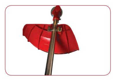
Locate the guard on to the lower shaft using the 2x screws provided.
