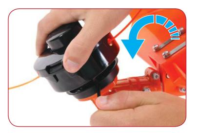
Lock the axle by placing the allen key inside the locating hole of the collar and wind the spool onto the thread by turning anti-clockwise.
