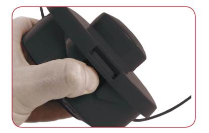
Open the spool by pressing one of the two clips to loosen the cover. Once loose firmly press the second clip and remove the spool cartridge from inside the housing.
