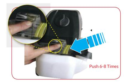
Prime the carburettor by repeatedly pressing the bulb located underneath the air filter housing Push 6-8 Times.
