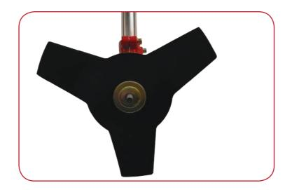
Install washer "B" as illustrated above to secure the blade to the shaft.
