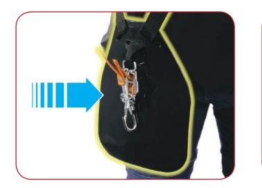
Ensure the thigh pad is located in the correct position so it protects you fully from pres sure points created from contact with the machine during use.
