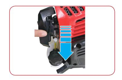
For warm engine starts open the choke by sliding the lever downwards.
