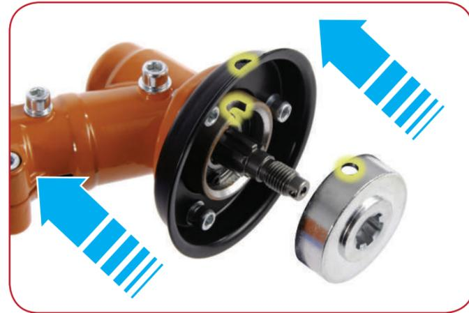
Align the holes on the collar, washer "A" and the axle. The areas highlighted above.
